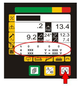
Press and release the RED pushbutton (4) the display will indicate the <u>next</u> page indicating **digital signals corresponding to the measurements of the other analog inputs**:
