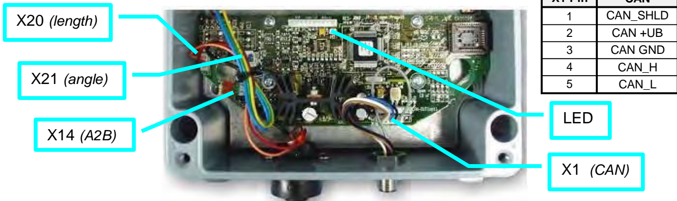
CAN-Bus electronics in angle sensor box.
