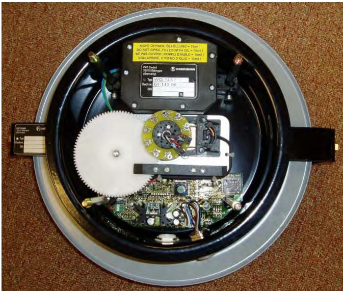
CAN-Bus electronics in cable reel.
