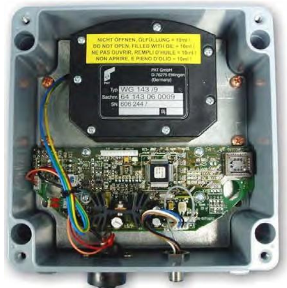
CAN-Bus electronics in angle sensor box.
