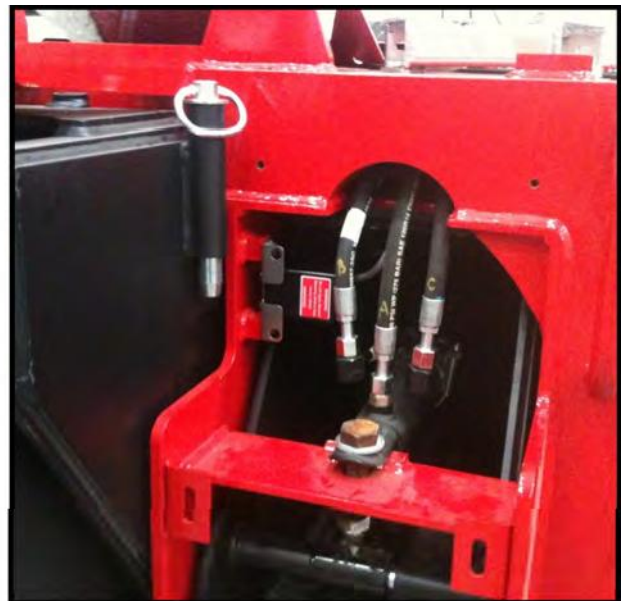
Sensor mounted in the outrigger box
