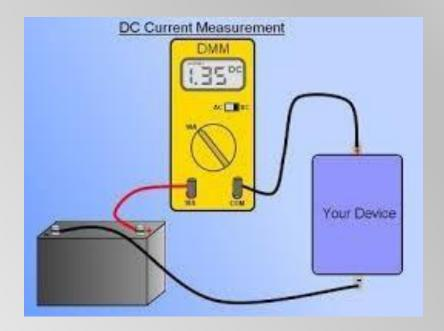
Once you have verified you have power to the Head Angle or Fly Angle Sensor(s) then you can measure the output of these sensors. The output voltage is 4 - 20 ma. These angle sensors are not CANBUS they are analog due to the length of the ATB cable. Since the connectors are sealed it will be easier to measure the current at the boom reel where the sensors are connected to the CANBUS Convertor board.
