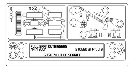
To view specific error codes, it is necessary to go into calibration mode.
