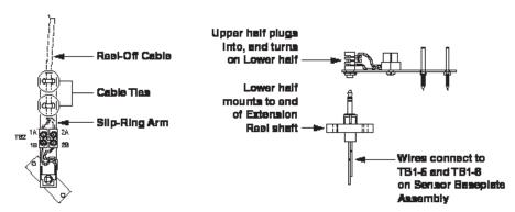
Failure of the slip-ring assembly will most likely result in a continuous ATB alarm. For information on testing and checking the slip-ring assembly, refer to the Anti-Two-Block on page 14.
