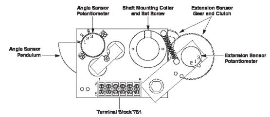
The terminal block (TB1), mounted on the assembly, provides wiring connection for all internal parts of the reeling drum, and the signal cable connecting the reel to the system computer. Most electrical diagnosis of the boom sensors may be made at this terminal block.
