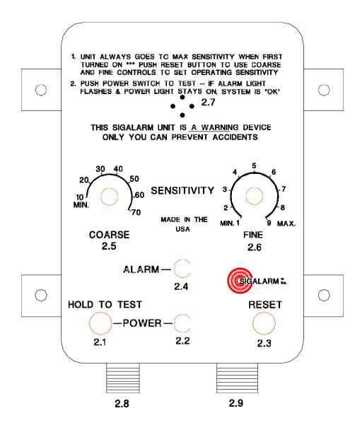
**HOLD TO TEST BUTTON** - allows the operator to test the entire system by pushing and holding down this button. This button then checks the entire system, if the green power light stays on, external horn sounds, internal buzzer works, and red light flashes the system is fully functional. If any of these are not working contact your supervisor and fix prior to use. If any of these fail there is either a break in the antenna, a jumper pin problem, or there is an internal failure.
