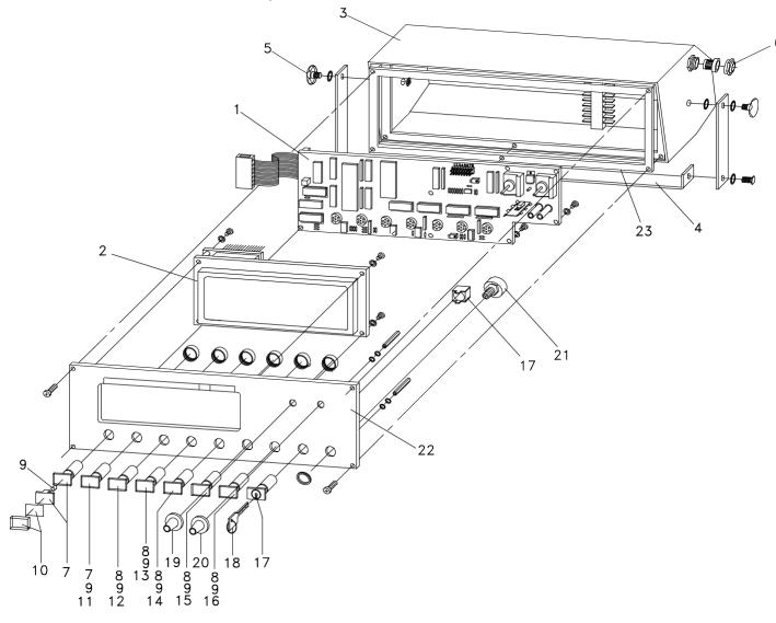
To change DS150/0008 (12V) to DS150/0012 (24V) a jumer wire must be soldered on main board, J3 added, and the ligth bulbs changed. When ordering spare part please specify 12 or 24 volt machine.
