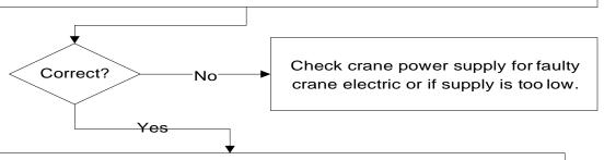
Measure voltage on the connection board between X1:30 (+12/24V) and X1:33 (ground). This is an output voltage to the console.
