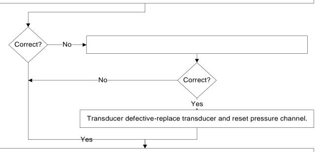
Connect wire No. 4 from transducer cables back to terminal X1:16 (rod side) and terminal X1:21(piston side). Without pressure in pipes or hydraulic pipes disconnected from transducer, check 0-point adjustment on connection board.
