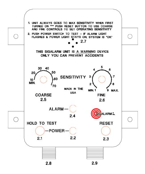
**HOLD TO TEST BUTTON** - allows the operator to test the entire system by pushing and holding down this button. This button then checks the entire system, if the green power light stays on, external horn sounds, internal buzzer works, and red light flashes the system is fully functional. If any of these are not working contact your supervisor and fix prior to use. If any of these fail there is either a break in the antenna, a jumper pin problem, or there is an internal failure.
