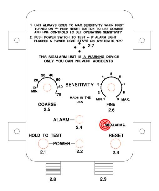
**HOLD TO TEST BUTTON** - allows the operator to test the entire system by pushing and holding down this button. This then checks the entire system. If the green power light stays on, external horn sounds, internal buzzer works, and red light flashes the system is fully functional. If any of these are not working contact your supervisor and fix prior to use. If any of these fail there is either a break in the antenna, a jumper pin problem, or there is an internal failure.
